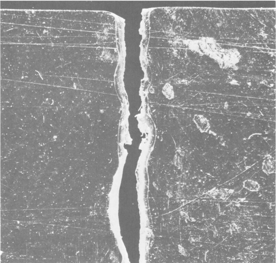
FIG. 11—Two consecutive sandwich bags related by individual surface scratches (magnification \times 10 ).
